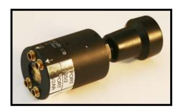
5/2 manually operated valve with 4mm push in ports and air override to reset. This valve can be used as a stand alone valve for operating a PTO or in conjunction with a separate solenoid valve to inhibit operation. This valve utilises our original eyeball indicator inside the knob which changes colour to red when valve and PTO are actuated.
